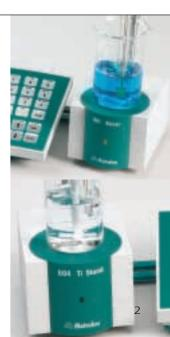
The 804 Ti-Stand with 802 Rod Stirrer offers an alternative way of stirring.
