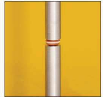
TA-TCA (P) (Tablet Coating Adhesion Fixture) Tablet 코팅의 점착력 측정 • Fixture Base Table 필요
